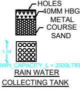
RAIN WATER COLLECTING TANK
