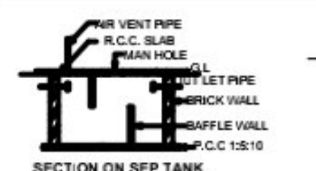
SECTION ON SEP.TANK
