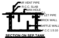
SECTION ON SEP.TANK
