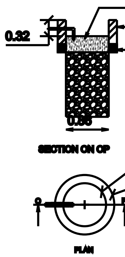
RAIN WATER PIT
