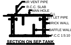
SECTION ON SEP TANK
