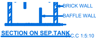
SECTION ON SEP.TANK
