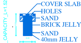
SECTION OF RAIN WATER COLLECTION TANK
