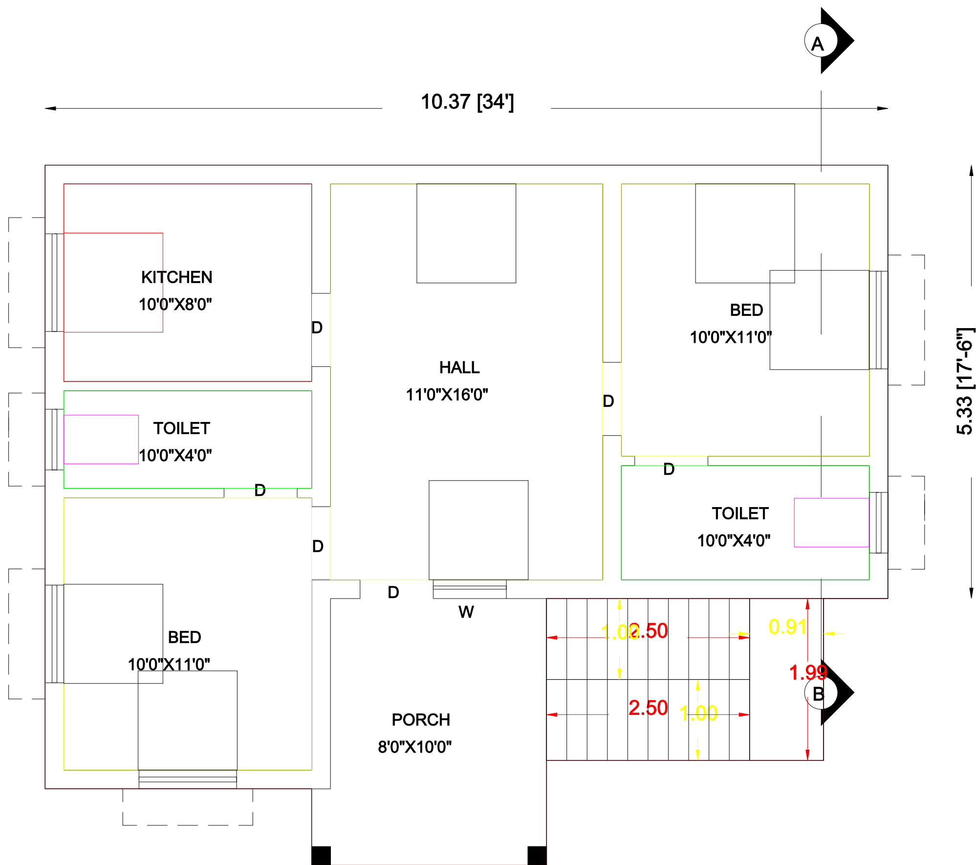
GROUND FLOOR PLAN
