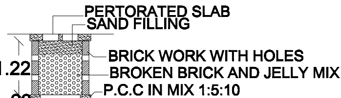
PERFORATED SLAB SAND FILLING
