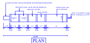
WASTE WATER RECYCLING SYSTEM
