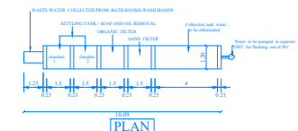
WASTE WATER RECYCLING SYSTEM PLAN
