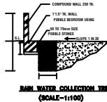
RAIN WATER COLLECTION TRENCH (SCALE-1:100)
