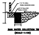
RAIN WATER COLLECTION TRENCH (SCALE-1:100)
