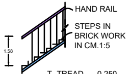
T- TREAD - 0.250 R- RISE - 0.175 WIDTH OF STAIR CASE - 0.910
