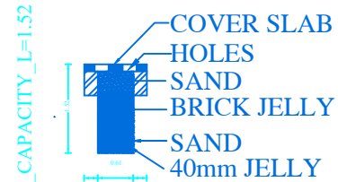
SECTION OF RAIN WATER COLLECTION TANK
