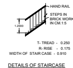
DETAILS OF STAIRCASE
