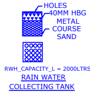
RAIN WATER COLLECTING TANK
