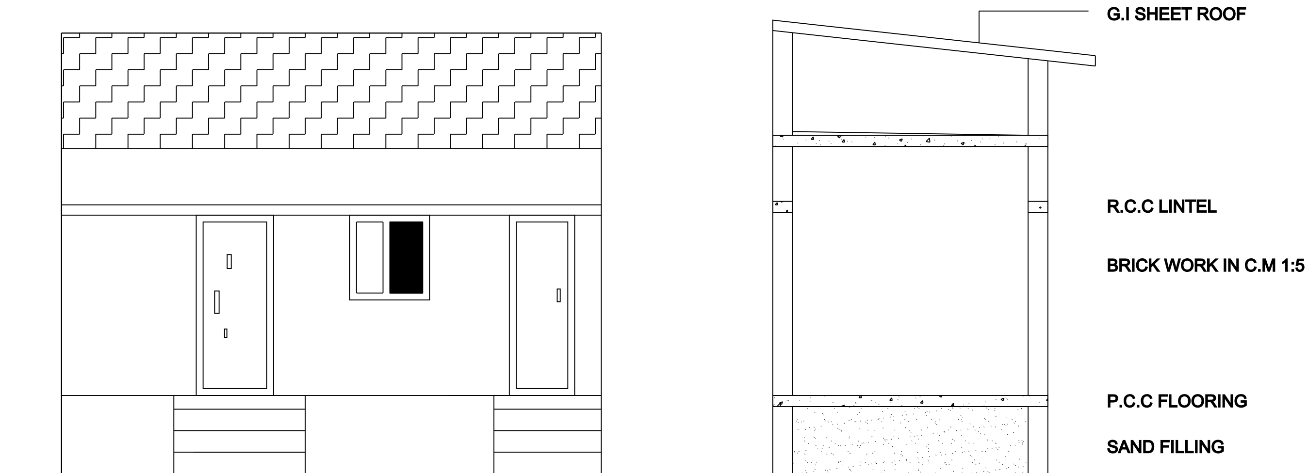
ELEVATION SECTION ON A-A
