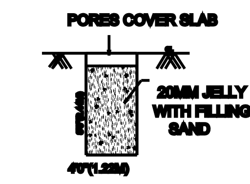
RAIN WATER HARVESTING UNIT
