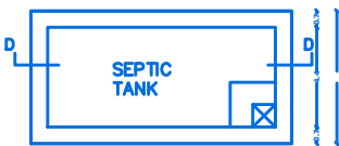
PLAN OF SEPTIC TANK SCALE 1"-2'-0"
