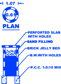
SECTION OF RAIN WATER COLLECTION TANK
