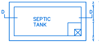
PLAN OF SEPTIC TANK SCALE 1"=2'0"
