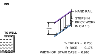
DETAILS OF STAIRCASE
