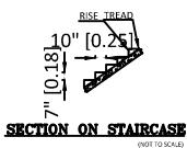
SECTION ON STAIRCASE
