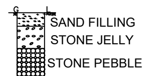
RAINWATER HARVESTING PIT
