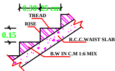
SECTION OF STAIRCASE
