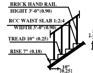
STAIRCASE DETAIL (SCALE 1:50)
