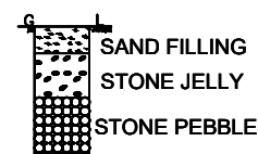
RAINWATER HARVESTING PIT
