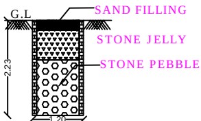
DETAILS OF RAIN WATER HARVESTING
