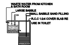
DETAILS OF RAIN WATER HARVESTING
