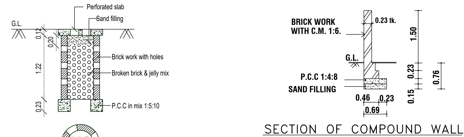
PERCOLATION PIT FOR 30 Sq. m. (Scale:- 1:50)
