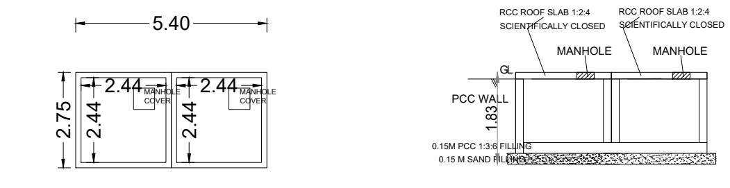
FIRE and RAIN WATER SUMP each 2.4 X 2.4X 1.83[ 10,00LTS CAPACITY]
