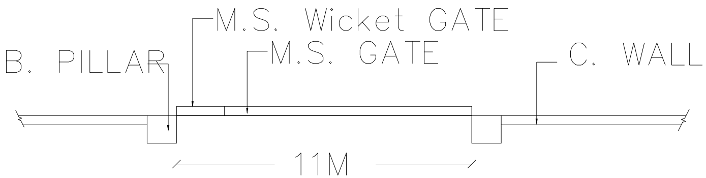
Plan Compound Wall & Gate Details
