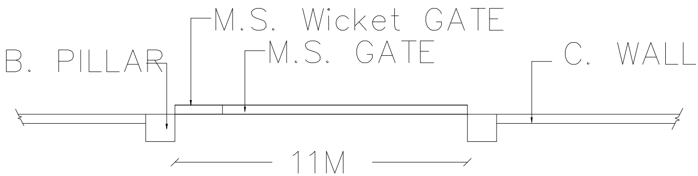
Plan Compound Wall & Gate Details
