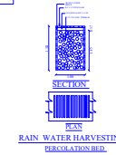
RAIN WATER HARVESTING PERCOLATION PIT
