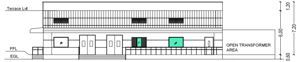
ELECTRICAL SUBSTATION BLOCK ELEVATION - 1
