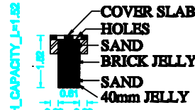
SECTION OF RAIN WATER COLLECTION TANK
