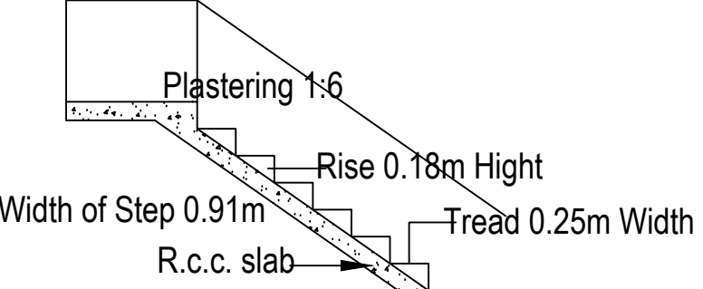
DETAILS OF STAIR CASE
