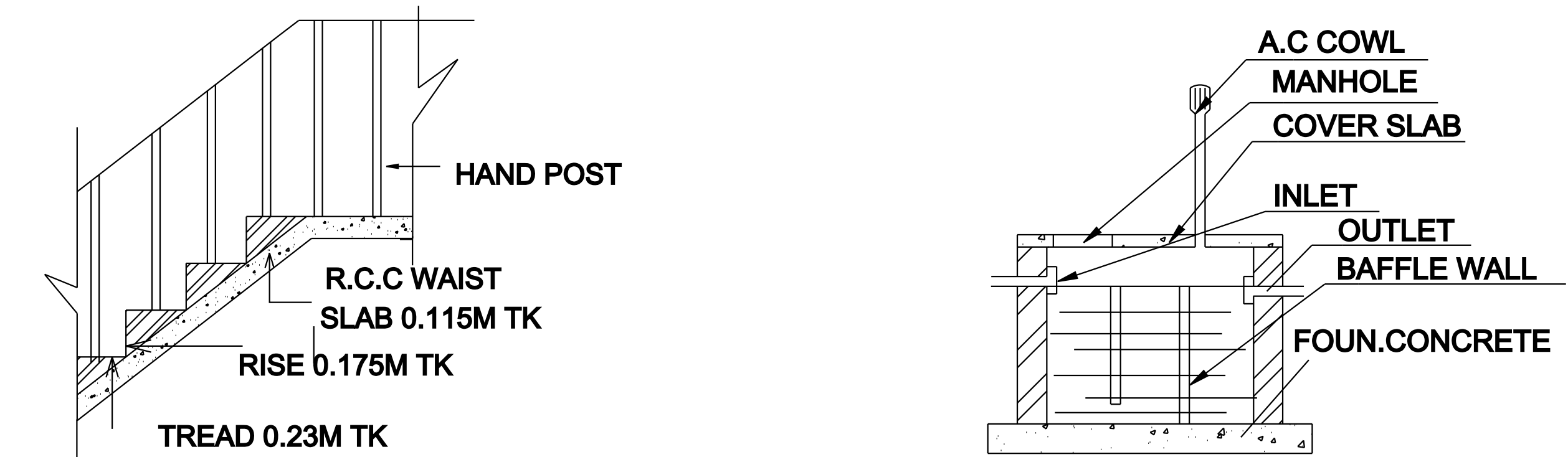
DETAILS OF STAIRCASE
